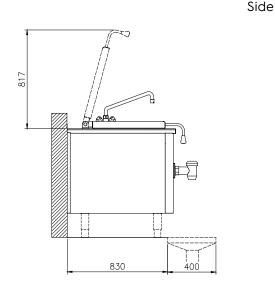
CWI1 Cold Water inlet 1 (cleaning) Electrical inlet (power) ΕI Hot water inlet
